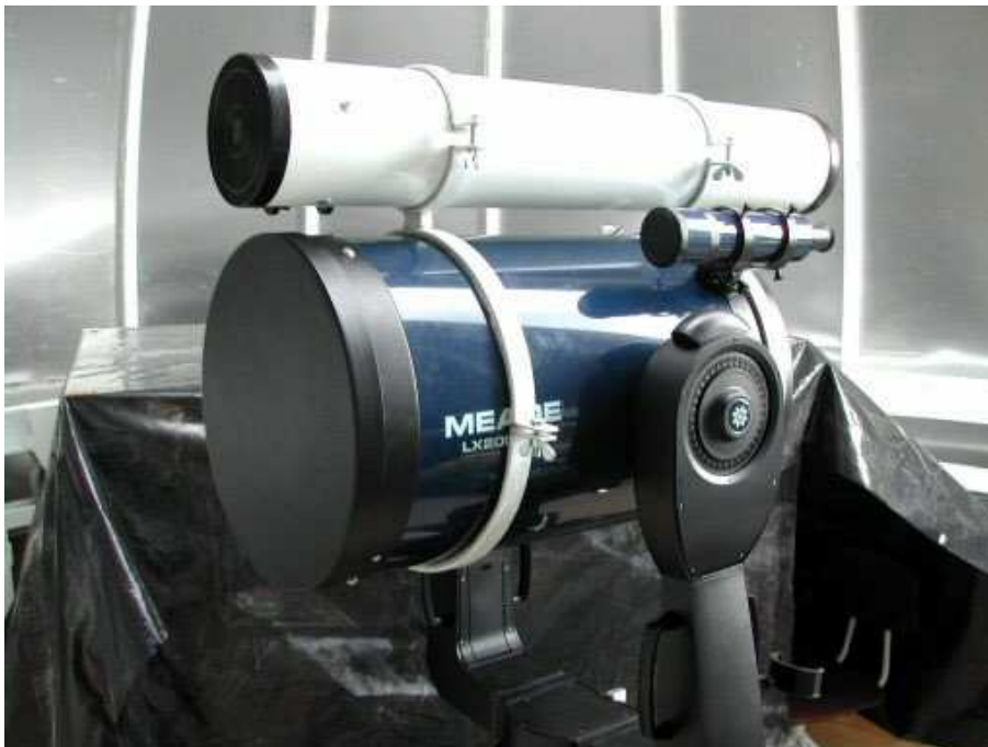
Figure 2.1: 12 inch Meade telescope with TAL-1 mounted on the top of it.
